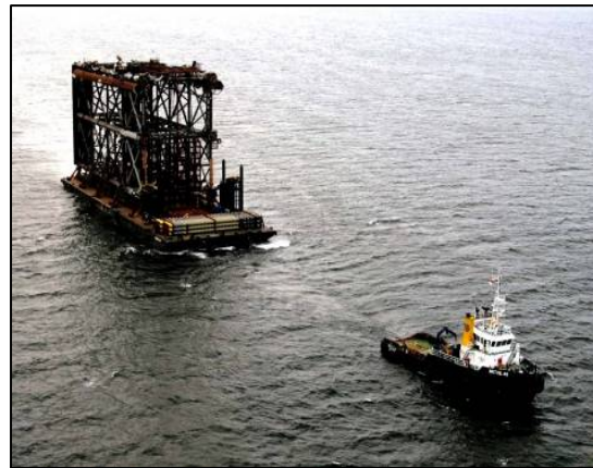
VR-B Jacket Being Shipped to Tangguh Site
